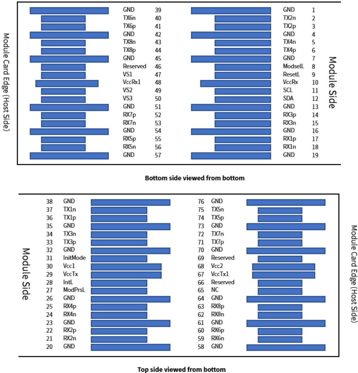
Figure 1 – QSFP-DD Compliant 76-pin connector (per QSFP-DD MSA)
